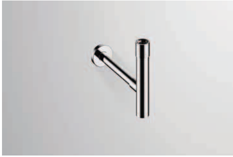
Bottle trap, w/h/d 45/297/370 mm, chrome-plated, 1 1/4" connection thread, immersion tube, adjustable in height from 135 to 205 mm, adjustable depth from 90 to 370 mm
